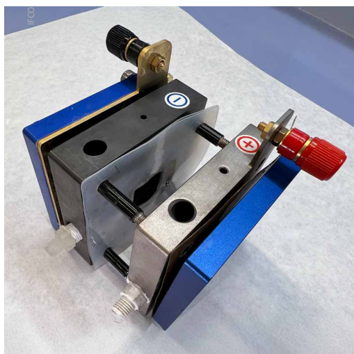
PEM water electrolyzer employed in the study
